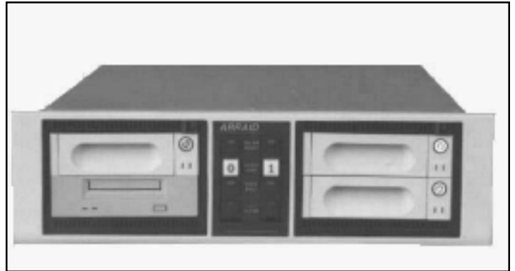
Dual Rack Mount AEM-1 with Tape Backup (l) and Disk to Disk Copy (r).
