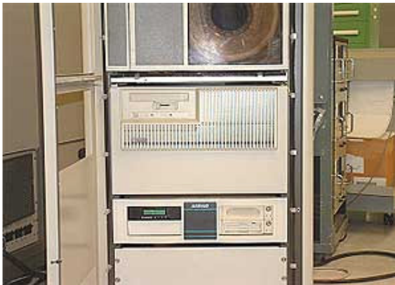
The AEM-8 replaces the 7914 in this radar ATE system at Hill AFB. (From top) HP 7970E tape drive, HP 7914R, and AEM-8 HP-IB Emulation System.
